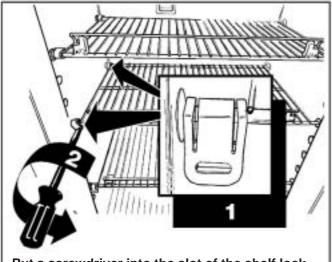
Put a screwdriver into the slot of the shelf lock. Turn the screwdriver counterclockwise. Remove the shelf locks from the wire shelf.
